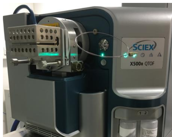
Figure 2: Schematic of the Thermal Extraction Ionization Source (TEIS). (Top) This source sits in front of the MS orifice and consists of two heated blocks, transfer line and location of the APCI needle. This configuration provides real-time peak detection and direct sample introduction. The bottom pane shows the source coupled to the SCIEX X500R QTOF System.
